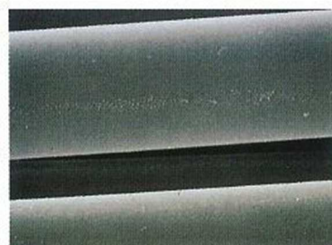
Held at 80°C for 200 hours in saturated cement solution
