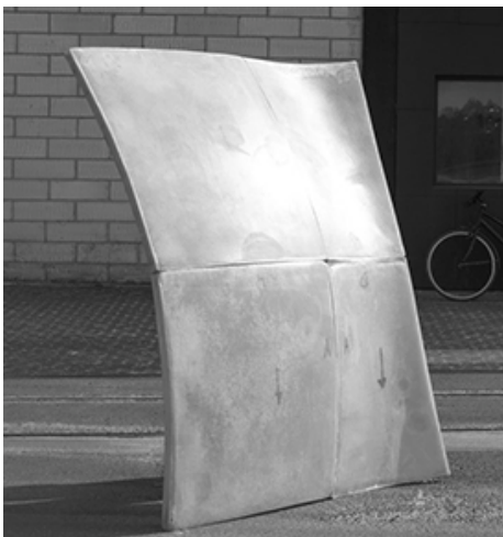
Figure 11 Thin-walled elements made on a flexible table.
