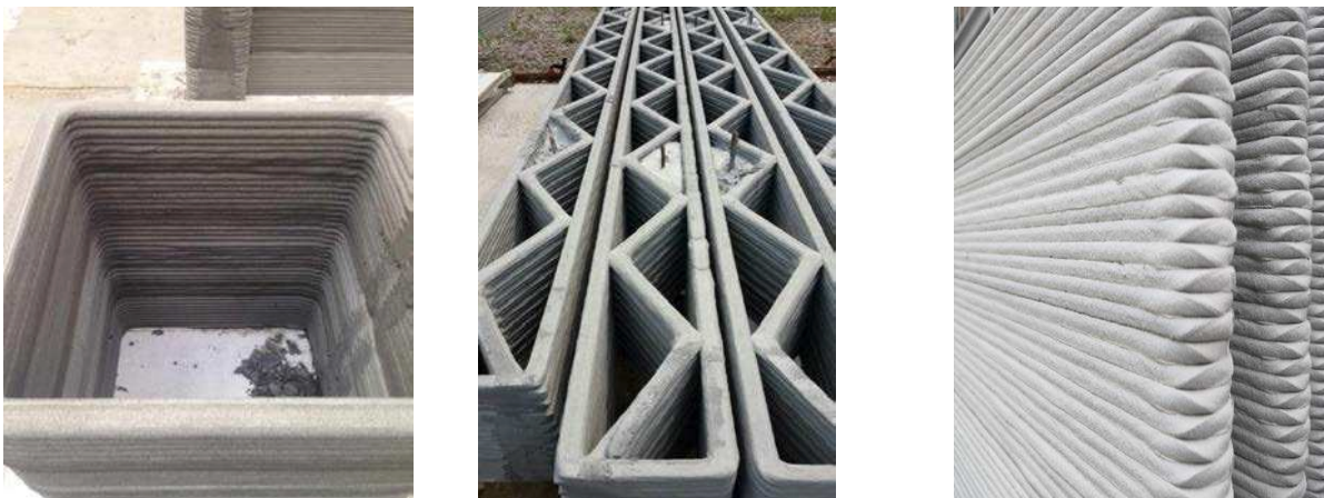
Figure 5. Various printed building elements
