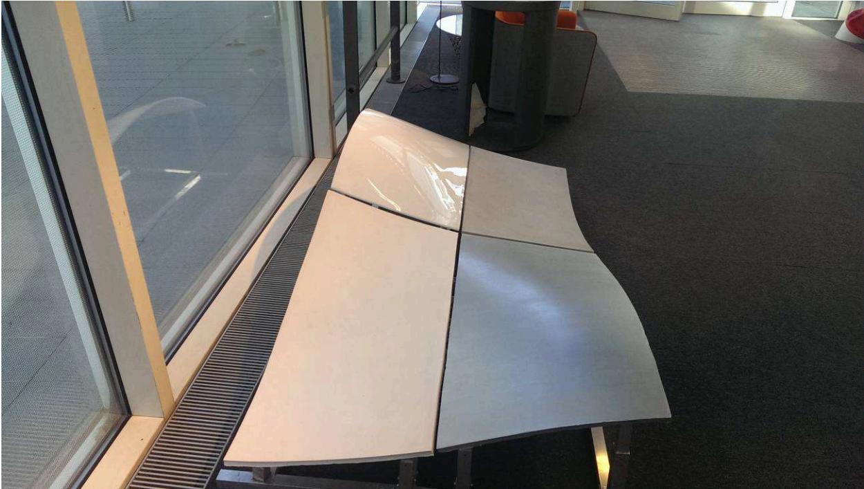
Figure 7. Exhibition panels at Foster+Partners made from GFRG, GFRC and Acrylic (1000x2200 mm).
