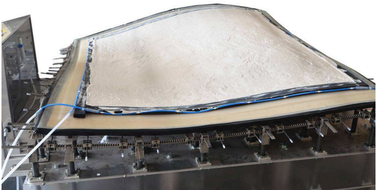
Figure 3. Casting of a double curved fiber reinforced concrete panel ( www.adapa.dk ).
