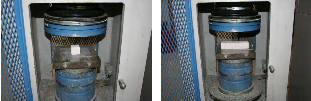
Figure 4. Compression tests and specimens used for compression tests
