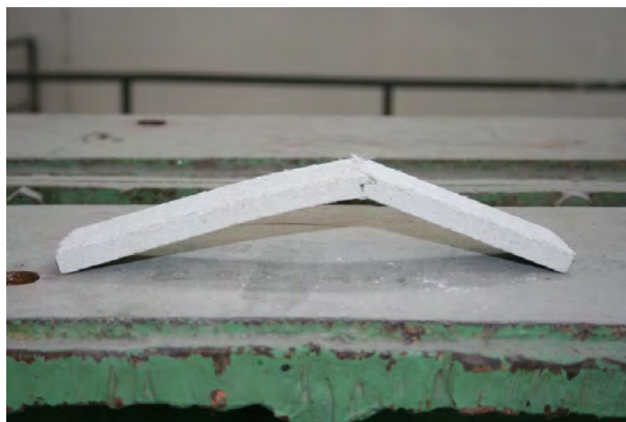
Figure 5. Bending tests and appearance of a specimen after test
