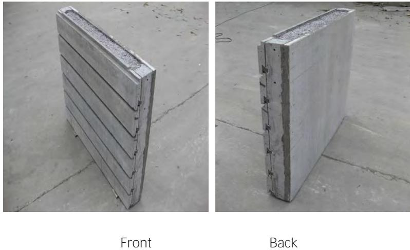
**Figure 13 External wall sample**
