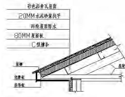
Figure 12 Roofing system
