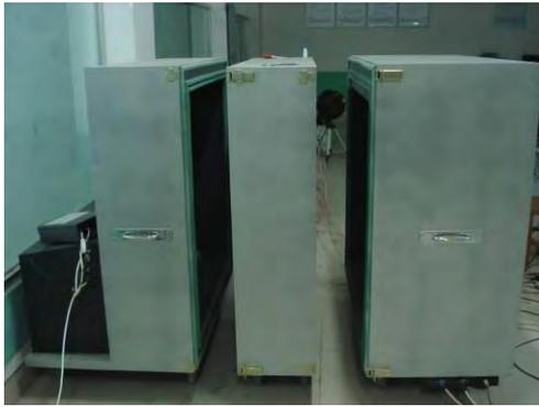
**Figure 15 Hot container, cool container and sample box**
