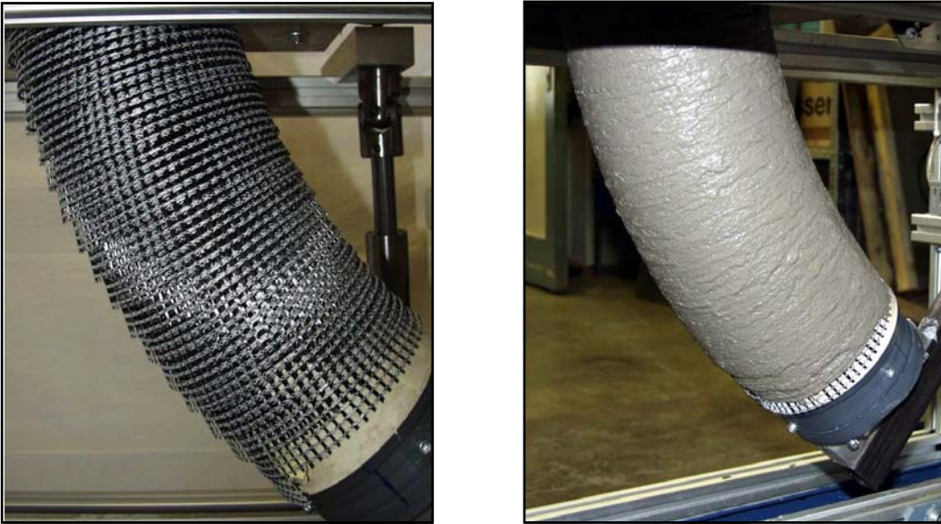
Fig. 2: Production of component at the Institute for Building Materials TU Dresden - (a) Reinforcing process - (b) Completed pipe elbow (right)
