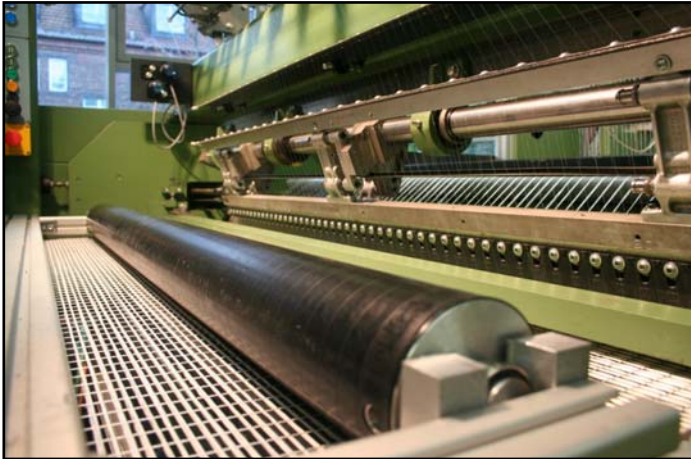
Fig. 5: Coating process on the multiaxial knitting machine
