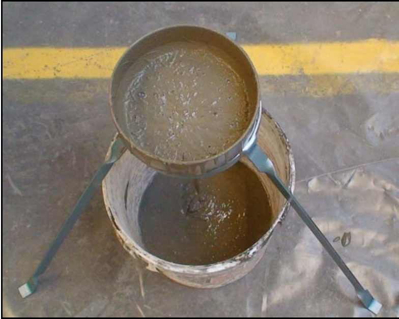
Figure 1. Fluidity test apparatus
