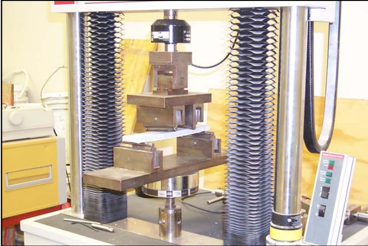
Figure 1 – Flexural Strength Test Rig
