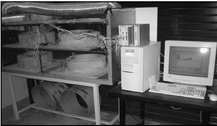
Fig. 3. Experimental set-up of shrinkage test and recording of strain gauge readings
