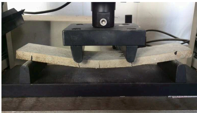
Figure 8. Multiple cracks of GRC sample
