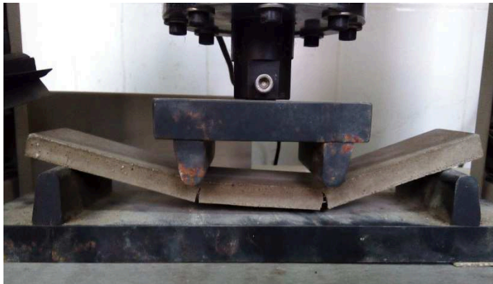
Figure7. Double cracks of GRC sample
