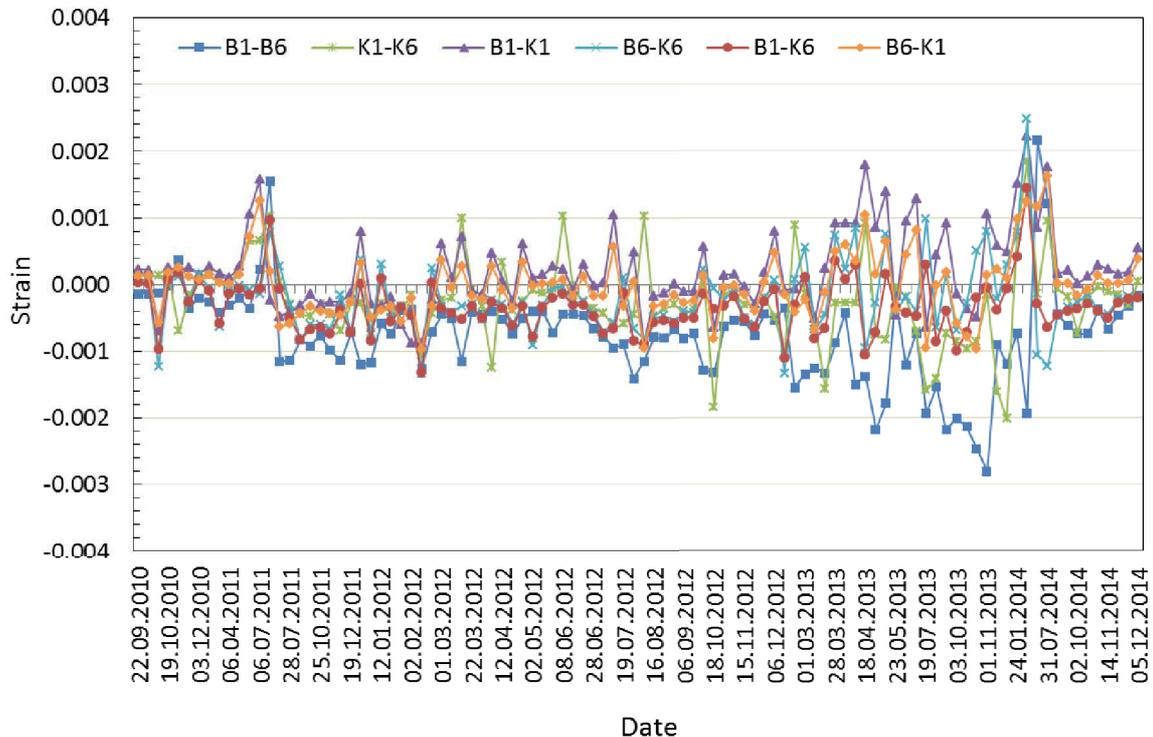
**Figure 8.** The evolution of strain by time for PN1 façade panel
