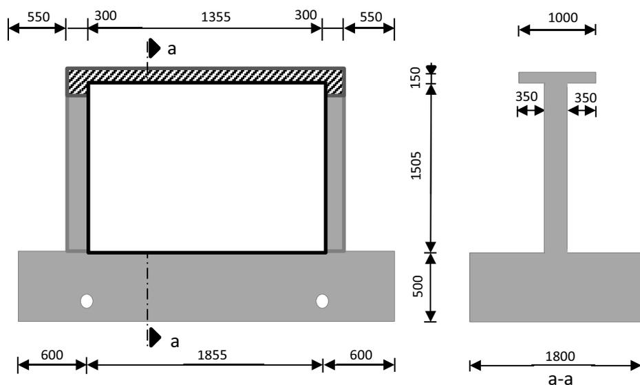
Figure 2. The appearance of the reinforced concrete frame (all dimensions in mm).
