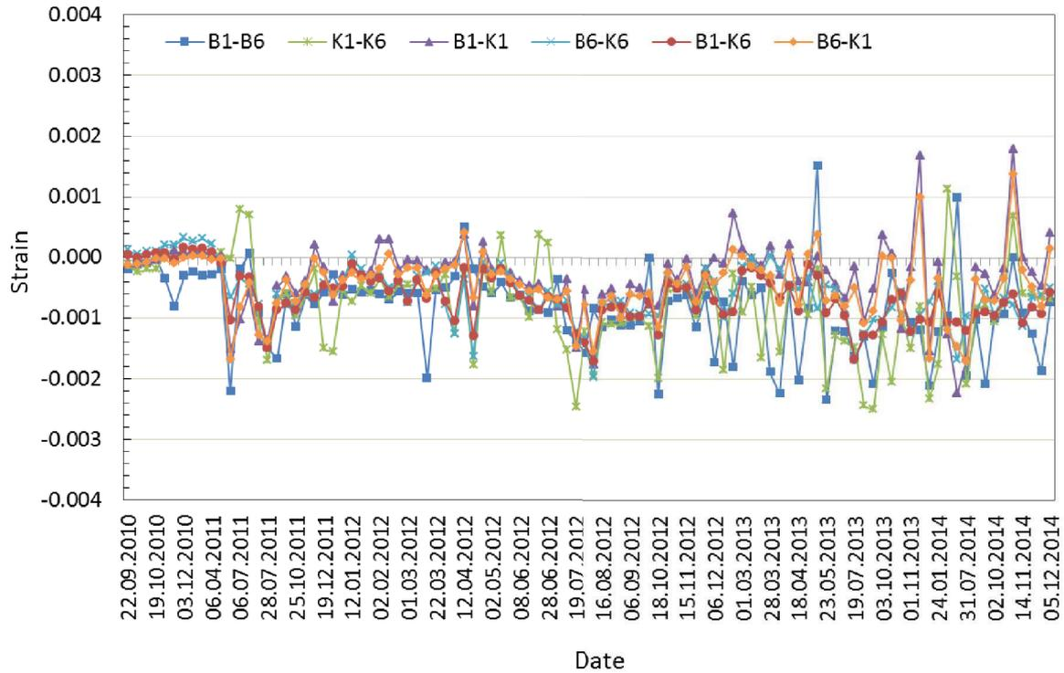
**Figure 9.** The evolution of strain by time for PN2 façade panel
