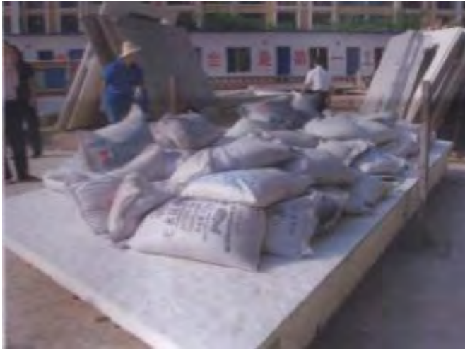
Fig.5 Field testing of a GRC sandwich panel
