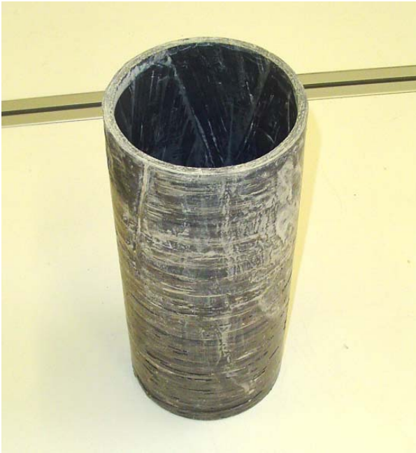
Figure 7: Specimen to be filled with concrete
