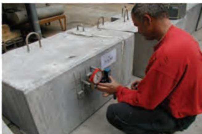
Figure 7 - Bonding strength test on a part of the test cornice Figure 8 - Specimen after a bonding strength test
