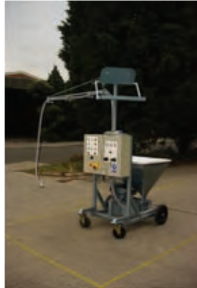
Figure 2 - Premix spray station
