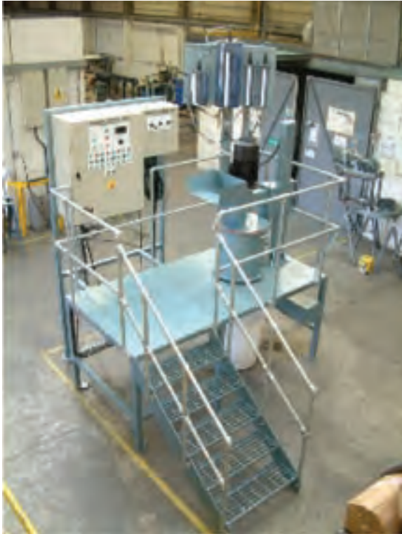
Figure 1 - Variable-speed mixer with water, polymer and admixture dispensing systems
